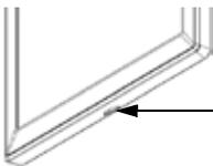
FIG. 24 The USB charging socket is located at the bottom edge of the display.
