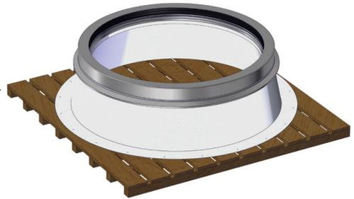
*Glass skylights of the FE series will be delivered already completely pre-assembled onto our curb. The skylights will be therefore packed on a wooden crate. The bottom of the wooden crate is designed with square timbers and can be transported with a forklift truck. Lifting up the skylights to the roof should be done including the wooden crate. For safety reasons, the skylights should kept as long as possible inside the wooden crate.*
