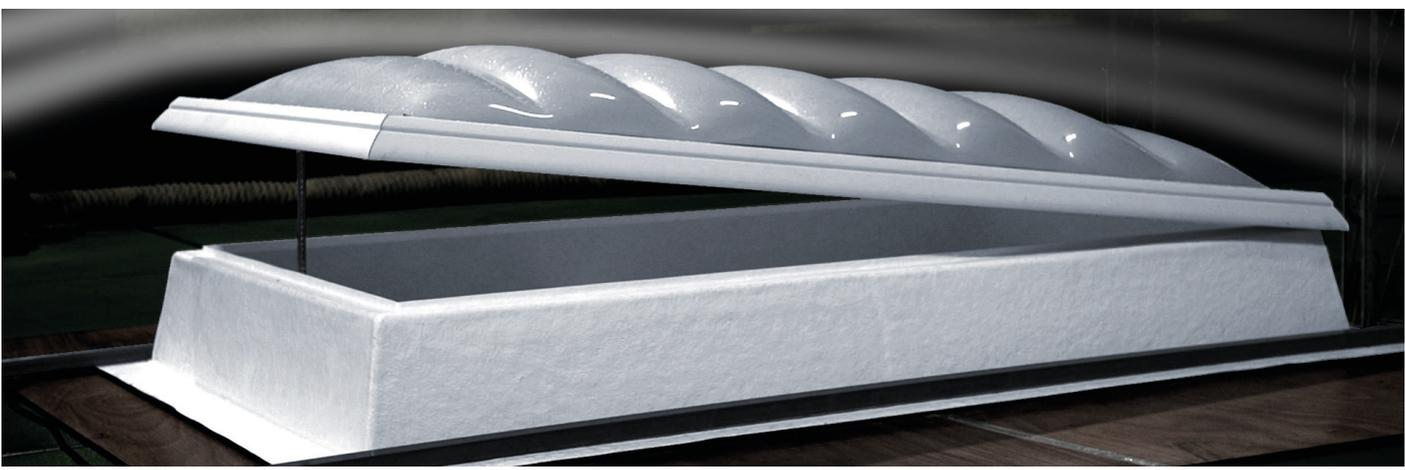
Rooflight F100 W in the extreme weather test in the wind tunnel
