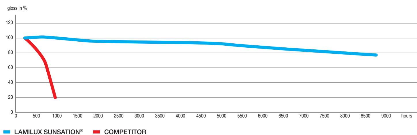
Artificial wetahering according to DIN EN ISO 4892- 2: color change  $\Delta E$  over time in % (9000 hours  $\approx$  15-20 years real time weathering central Europe)
