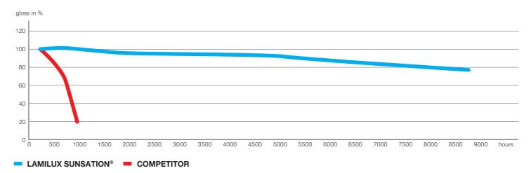
Artificial wetahering according to DIN EN ISO 4892- 2: color change  $\Delta$  E over time in %(9000 hours ≈ 15-20 years real time weathering central Europe)
