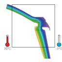
Example: isothermal characteristic of a 10° isothermal line, shown in red, in a triple-glazed LAMILUX CI System Rooflight Dome F100 under specified boundary conditions. The isothermal line is featured as a steady outline within the structure - the risk of condensation is minimised.
