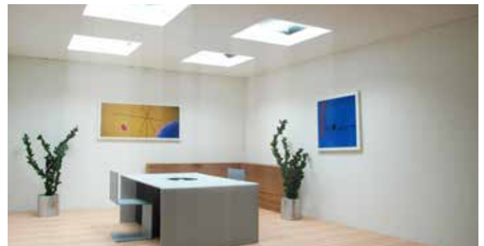
Highly reflective shaft - maximum DQ at user level approx. 8%
