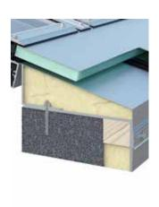
Installation on concrete upstand
