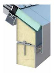
Installation on steel sheet upstand
