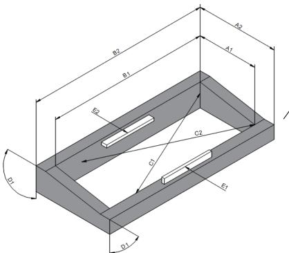
the upstand must be designed to be load-bearing all around and can safely absorb all vertical loads and horizontal spreading forces.
